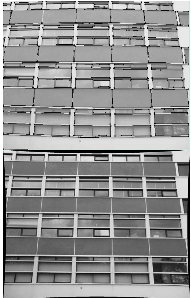
Figure 2: First wide-angle image with extracted lines (top) and corrected for radial lens distortion (bottom).
