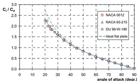
Figure 5: The lift drag ratio of three airfoils with varying thickness at high angles of attack compared to ideal flat plate theory.
