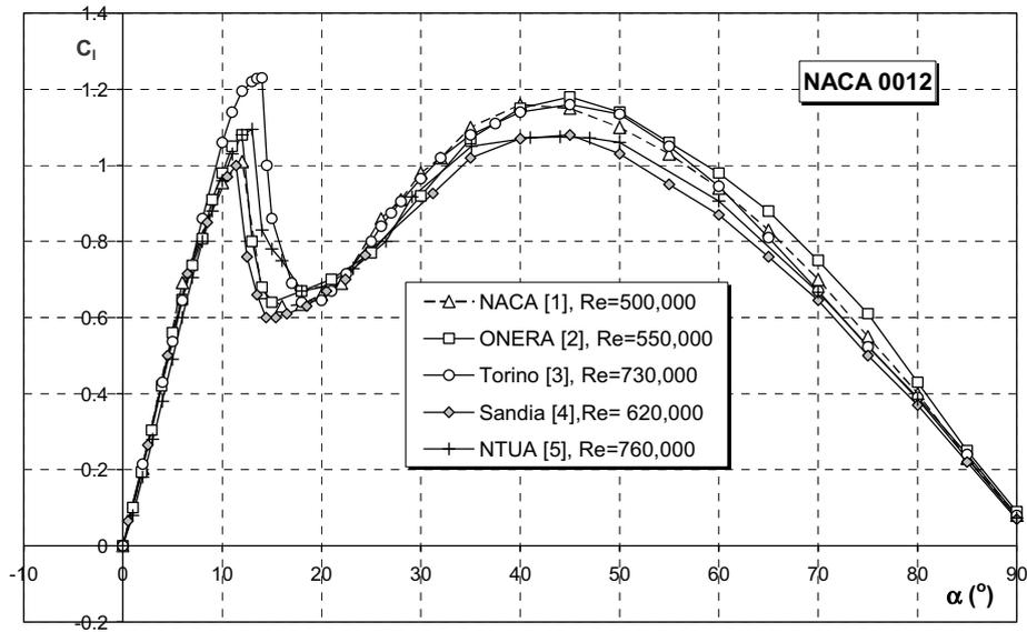
Figure 1: Measured two-dimensional aerodynamic characteristics of airfoil NACA 0012
